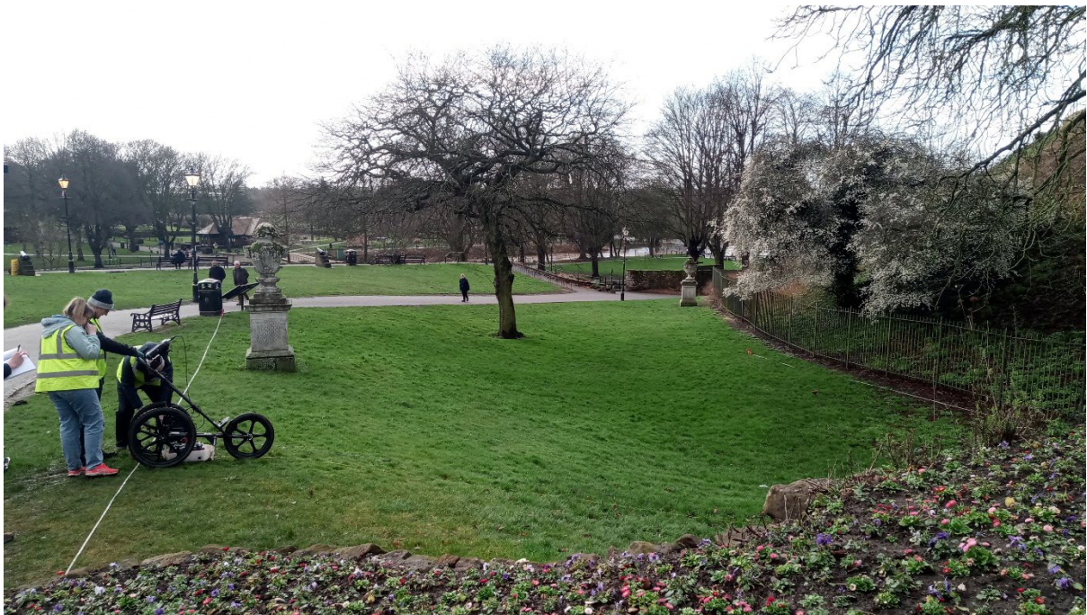
Ground Penetrating Radar survey being undertaken at Tamworth Castle
